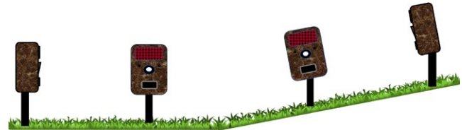
FIGURE 5 For maximum detections, camera traps must be angled to match the slope of the ground [Colour figure can be viewed at wileyonlinelibrary.com ]
